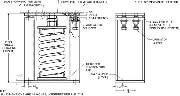
BOLT OR WELD EQUIPMENT SUPPORT BEAM TO MOUNT
